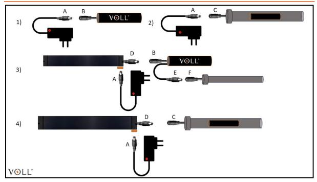
A = DC3.5X1.35-M; B = DC3.5X1.35-F; C = DC3.5X1.35-F; D = DC3.5X1.35-M; E = DC5.5X2.1-M; F = DC5.5X2.1-M.
