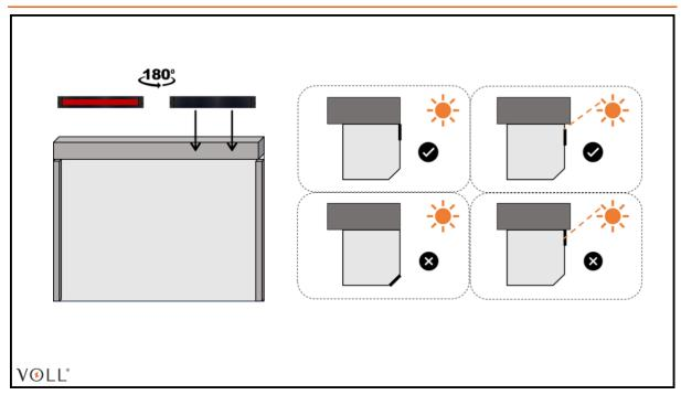
The solar panel is attached by means of a self-adhesive adhesive strip, this is done on the flat and cleaned surface of the housing or shade of the awning.
